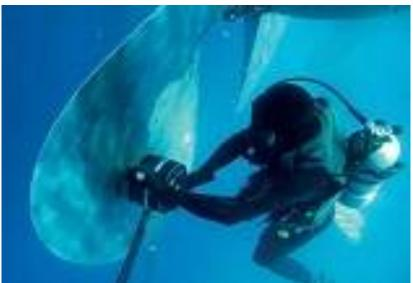
There are various methods of estimating the level of fouling on a propeller. These are the same methods used for general hull fouling. Most propeller efficiency conscious owners/operators schedule propeller polishing every six months or so; a less conscientious approach might result in propeller polishing once a year. The evidence is that keeping a propeller clean of anything more than a slime layer, and cleaning before a hard, calcare-
