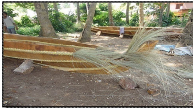
Figure 1: Representation of stitched boats showing X-pattern stitching in longitudinal and transverse direction.
