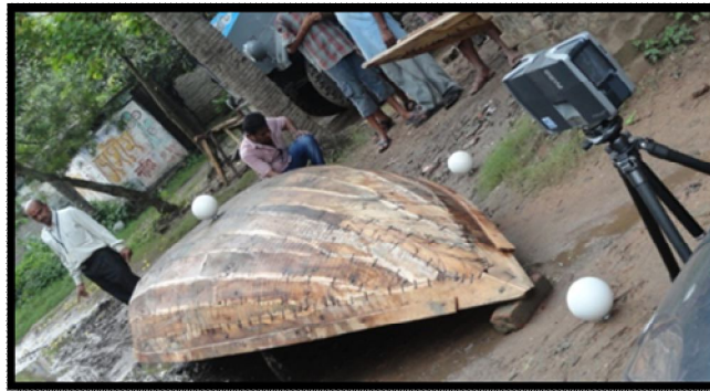
Figure 2: Representation of Nailed Plank built boat "DINGHY", West Bengal and taking scan of craft model using 3D laser scanner.
